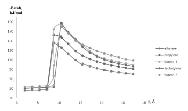
Stabilization becomes greatest with nanotube diameters from 9.52–12.23 Å. The maximum stabilizing effect is observed at 10.18 Å.
