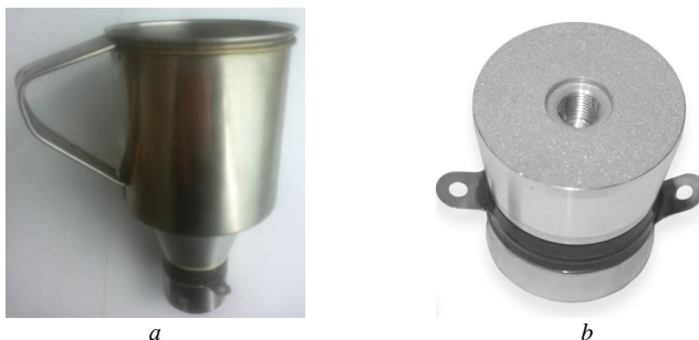
Fig. 1. Laboratory stand ( a ) for intensification of chemical processes based on Langevin's radiator ( b )
