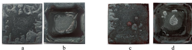
Fig. 1. The influence of salty (a, b) and desalted (c, d) coal on morphology of metal surfaces
